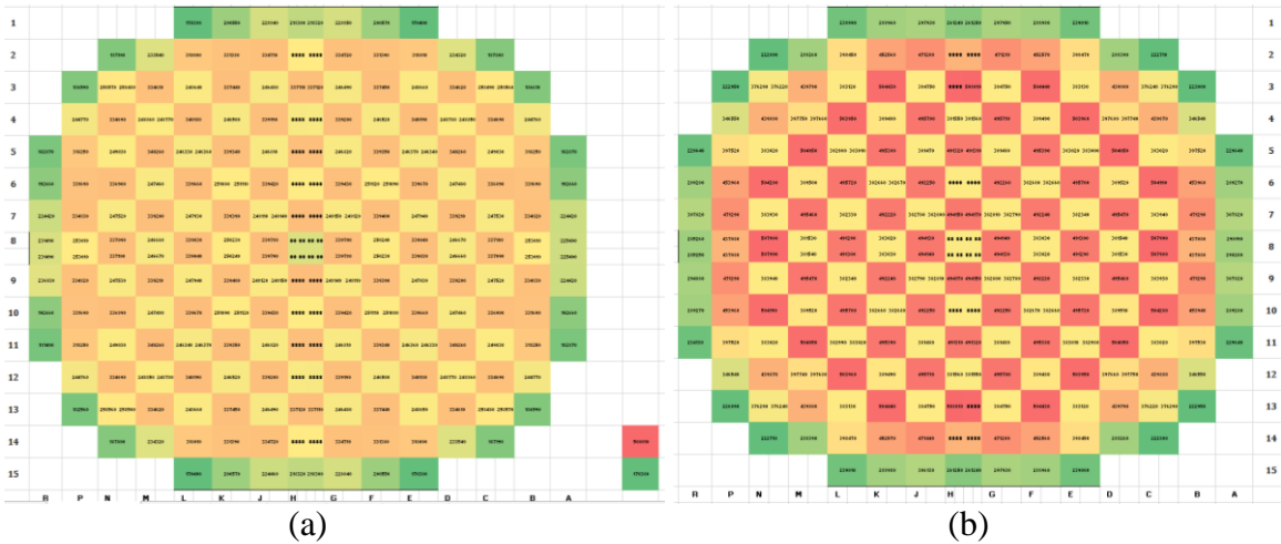
Figure 5.47: Fuel stored energy in each assembly for a (a) \text{U}_3\text{Si}_2/\text{SiC} fueled core, (b) \text{UO}_2/\text{SiC} fueled core
